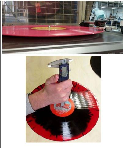
Warping must not affect the playing of record on a turntable. The tolerance for standard one colour record is max. 2mm.
